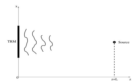
Figure 2. The time reversal procedure. A source with central wavelength  $\lambda_0$  emits a pulse. The transmitted field is recorded, stored and time reversed at the mirror of size a at a distance L away, and then sent back toward the source point. There it refocuses on the spot size,  $\rho_{\rm tr}$ , described by (75) when the medium is homogeneous. Medium heterogeneity typically enhances the refocusing resolution.
