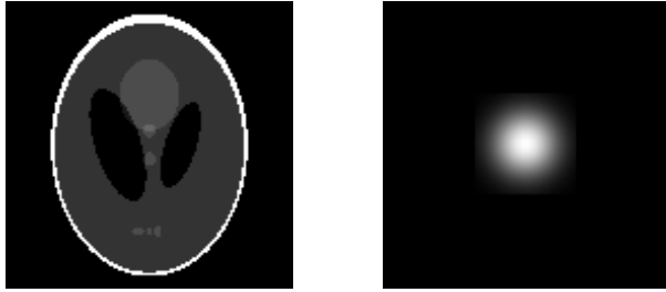
Figure 3: Left: Original image; Right: Gaussian filter in Fourier domain. The support of the filter is 45 \times 45 and hence m = 45^2 = 2025, n = 128^2, p = 32 .
