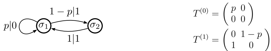
FIG. 1: A hidden Markov model (the \epsilon -machine) for the Even Process. The machine has two internal states \mathcal{S} = \{\sigma_1, \sigma_2\} , a two symbol alphabet \mathcal{X} = \{0, 1\} , and a single parameter p \in (0, 1) that controls the transition probabilities. The graphical representation is presented on the left, with the corresponding transition matrices on the right. In the graphical representation, transitions denote the probability p of generating symbol x as p|x .
