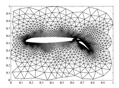
In a two-dimensional model, a triangular grid surrounds a cross section of the wing and flaps. The partial differential equations are nonlinear and involve several unknowns, including hydrodynamic pressure and two components of velocity. Each step of the nonlinear iteration requires the solution of a sparse linear system of equations. Since both the connectivity and the geometric location of the grid points are known, the gplot function can produce the graph shown above.
