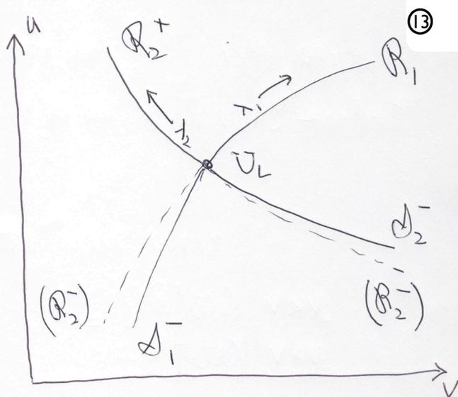
Principle: Pick out the shock curves  $\Delta_2^-$  that move in the directions of  $R_2$  in which  $\lambda$  decreases, since there are directions in which we cannot obtain simple wave solutions
