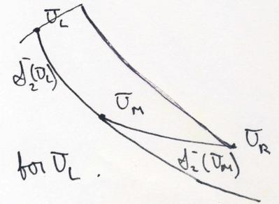
Theorem. The interaction of two 2-shocks produces a 1-rarefaction wave and a 2-shock wave.
