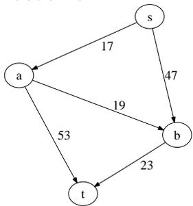
$$\begin{aligned} \min \quad & 17x_{sa} + 47x_{sb} + 19x_{ab} + 53x_{at} + 23x_{bt} \\ \text{subject to} \quad & x_{sa} = x_{ab} + x_{at} \\ & x_{sb} + x_{ab} = x_{bt} \\ & x_{ij} \in \{0, 1\}, \text{ for all } i, j \end{aligned}$$
