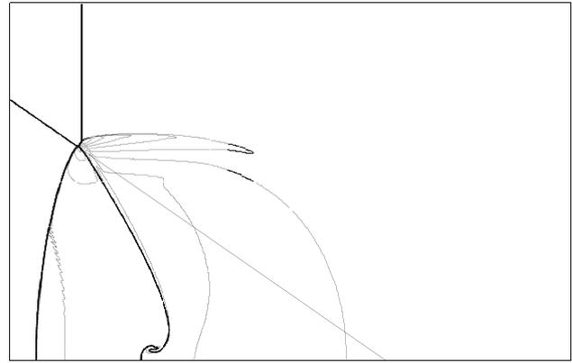
**Fig. 26** Contour plot of  $\log \rho$  for a PCMR in Air/CH<sub>4</sub> with  $\xi_i = 0.30$  and  $\alpha_i = 55^\circ$
