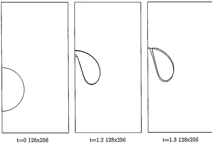
**FIG. 11.** Spherical gas bubble in liquid. Density ratio 816 : 1,  $We = 200$ . Results computed using the volume-of-fluid method (thin contour) are compared to results computed using the boundary integral method (thick contour).
