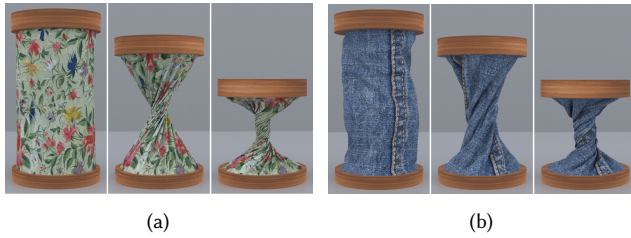
Fig. 4. Twisting Orthotropic Model. Using the data-driven model of Clyde et al. [2017] for woven materials, the characteristic wrinkling of silk (left) and denim (right) is obtained. Our method naturally resolves the many self-collisions induced by the twisting boundary conditions.
