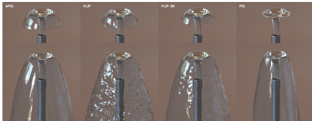
Figure 5: Here we compare the methods on a fountain simulation of free-surface flow. The top row shows that while APIC and FLIP are the least dissipative in the initial stages, the FLIP surface is already displaying a noisy leading edge relative to the more smoothly resolved APIC. The bottom row shows that the entire surface of the fountain becomes noisy with FLIP in the later stages. ©Disney.
