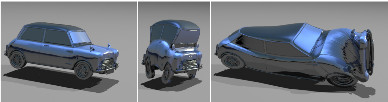
Fig. 26: Dynamic simulation of a soft elastic car model deforming under kinematic constraints, using linear elasticity. Resolution: 43K cells.
