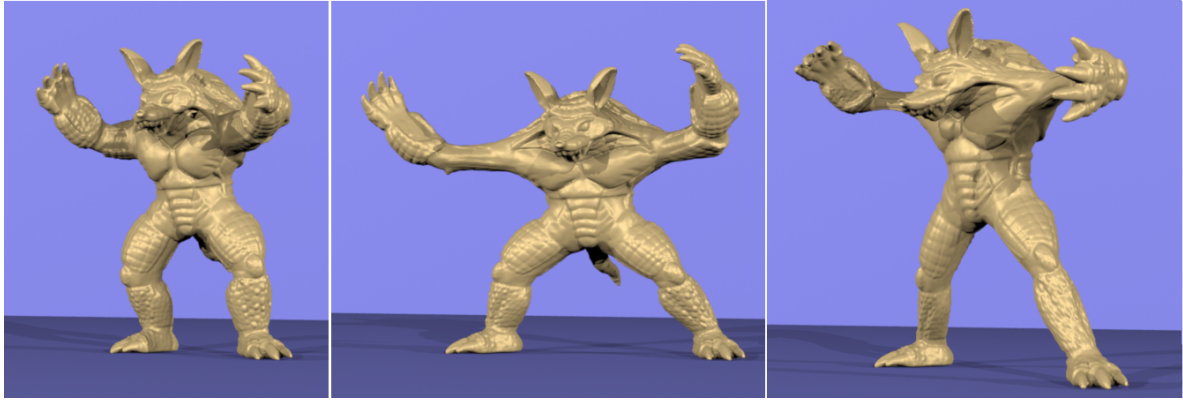
Fig. 24: Quasistatic simulation of armadillo model with co-rotational linear elasticity. Resolution: 302K cells.
