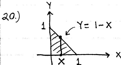
$$\begin{aligned} \text{Vol} &= \int_0^1 \int_0^{1-x} (1-x-y) dy dx \\ &= \int_0^1 (y - xy - \frac{1}{2}y^2) \Big|_{y=0}^{y=1-x} dx \end{aligned}$$
