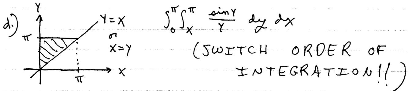
$$= \int_0^\pi \int_0^y \frac{\sin y}{y} dx dy = \int_0^\pi \left( \frac{\sin y}{y} \cdot x \Big|_{x=0}^{x=y} \right) dy$$
