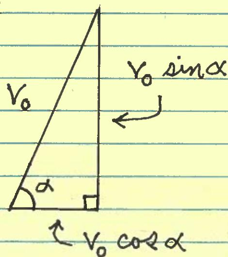
From Trigonometry we have the vertical and horizontal components of the initial velocity.
