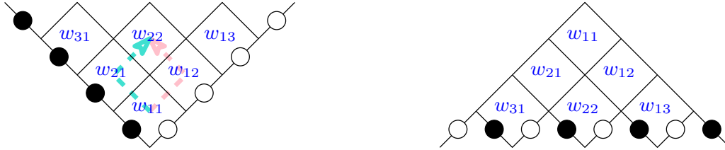
FIGURE 2. Left panel: a step initial condition in the TASEP corresponds to the wedge-type broken line interface. The shape of the interface after time t can be computed using last passage times: the time when a box (i, j) is added to the interface is L(i, j) . In particular, L(2, 2) = \max(w_{11} + w_{12} + w_{22}, w_{11} + w_{21} + w_{22}) . Right panel: by flipping the picture we can get the TASEP with a flat initial condition.
