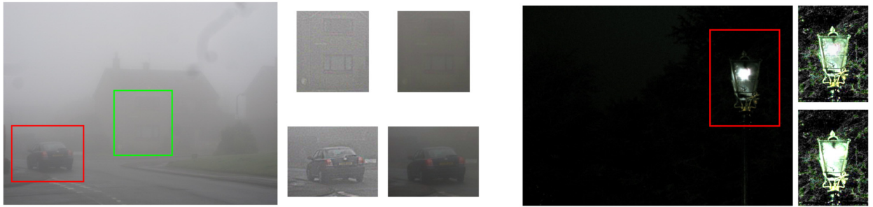
Fig. 16. Left group of images demonstrates image dehazing: results obtained with the approach presented in this paper (left) and results obtained with (He et al., 2011) (right). Right group of images demonstrates low light image enhancement: results obtained with the approach presented in this paper (top) and results obtained with (Guo et al., 2017) (bottom). These images are best seen on a computer screen.
