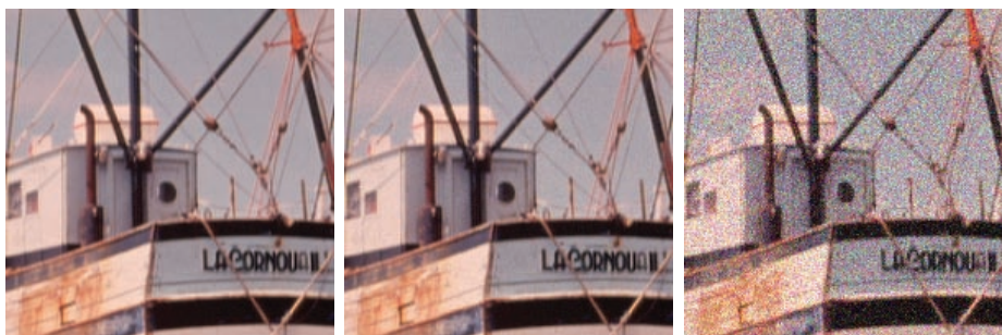
Fig. 1 A digital image with standard deviation 55, the same with noise added (standard deviation 3), the SNR therefore being equal to 18, and the same with SNR slightly larger than 2. In the second image, no alteration is visible. In the third, a conspicuous noise with standard deviation 25 has been added, but, surprisingly enough, all details of the original image still are visible.
