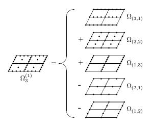
Figure 4.14. Combination technique for d = 2: combine coarse full grids  $\Omega_{\mathbf{l}}$ ,  $|\mathbf{l}|_1 \in \{n, n+1\}$ , with mesh widths  $2^{-l_1}$  and  $2^{-l_2}$  to get a sparse grid  $\Omega_n^{(1)}$ corresponding to  $V_n^{(1)}$ .
