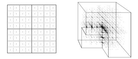
Figure 3.6. Sparse grids: regular example (left) and adaptive one (right).
