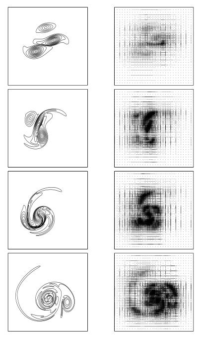
Figure 5.21. Isolines of  $\omega$  at t = 5, 10, 15, 35 (from top to bottom). Left: adaptive wavelet solver ( $\epsilon = 4 \cdot 10^{-4}$ ). Right: adaptive sparse grid.
