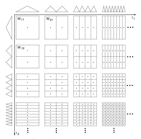
Figure 3.3. Scheme of subspaces for d = 2. Each square represents one subspace  $W_{\mathbf{l}}$  with its associated grid points. The supports of the corresponding basis functions have the same mesh size  $\mathbf{h}_{\mathbf{l}}$  and cover the domain  $\Omega$ .
