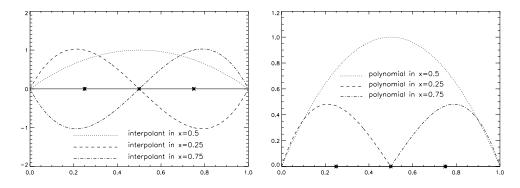
Figure 4.6. Hierarchical basis polynomials for p = 2 and p = 3 (different scaling for clarity): construction via hierarchical Lagrangian interpolation (left) and restriction to the respective hierarchical support (right).
