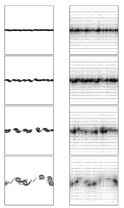
Figure 5.23. Isolines of the rotation for the values  $\{0.1, 0.2, 0.3, 0.5, 0.75, 1.0, \ldots, 2.25, 2.5\}$  at time t = 4, 8, 16, 36. Left: isolines of computed rotation. Right: adaptive sparse grid.
