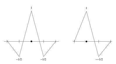
Figure 4.10. Non-orthogonal linear spline wavelet (left: interior; right: boundary).
