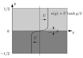
Figure 5.22. Velocity profile of the initial condition for the shear flow model problem. The thickness of the boundary layer is defined as  $\delta = 2U/\max_{u} |\partial_{u}u(y)|$ .
