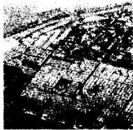
Fig. 10. Example of SAR data focused with proposed technique: area of Ventura (Los Angeles) is shown ( L band NASA DC-8 data taken in 1988). Dimensions: 3 Km in azimuth (horizontal) by 3 Km in slant range (vertical). Resolution: about 10 m in azimuth by 7 m in slant range (8 : 1 presuming).
