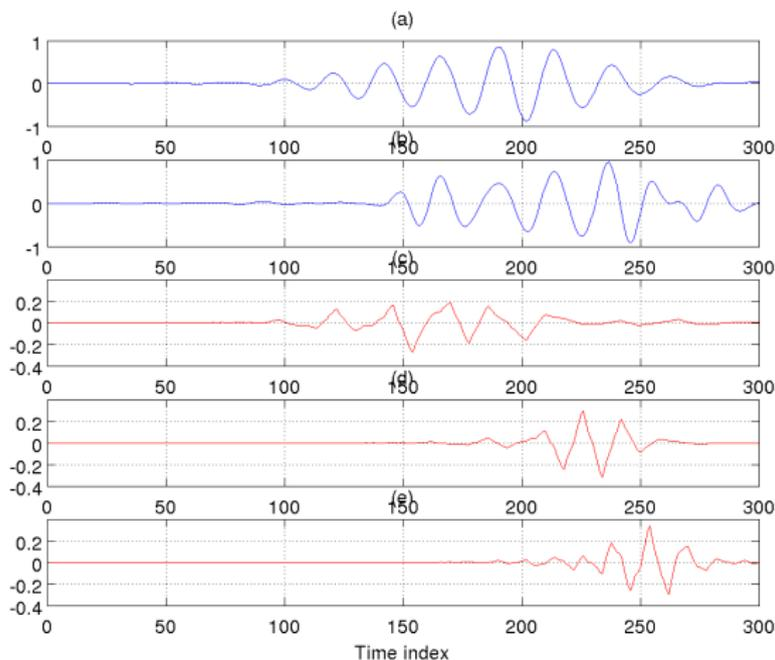
**Figure:** (a) Average C1 waveform; (b) Average S1 waveform; (c) The LDB vector #1 trained on (C1, S1); (d) The LDB vector #2 trained on (C1, S1); (e) The LDB vector #3 trained on (C1, S1).
