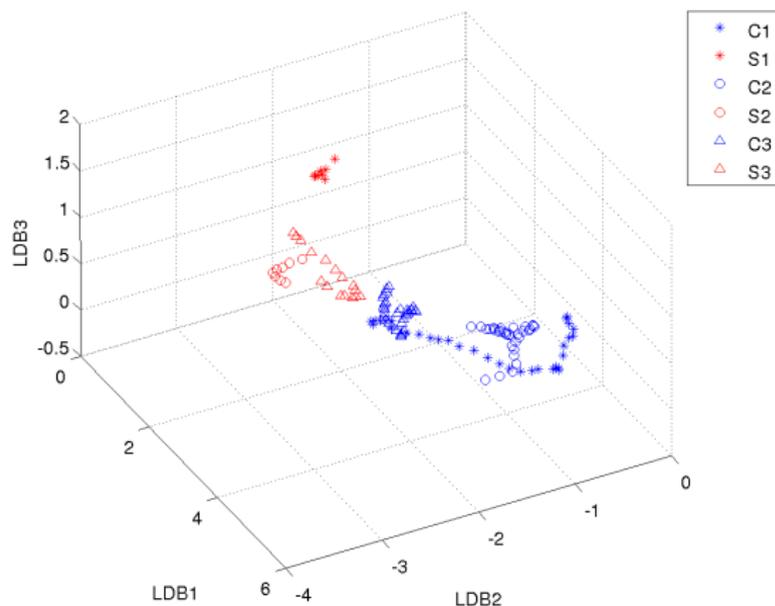
**Figure:** Extracted waveforms projected onto the top 3 LDB coordinates. Each point represents a single waveform. The LDB was computed on the (C1, S1) dataset.
