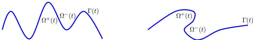
FIGURE 1. Two examples of the evolution of a vortex sheet \Gamma(t) by the Euler equations. The two fluid regions are denoted by \Omega^+(t) and \Omega^-(t) .
