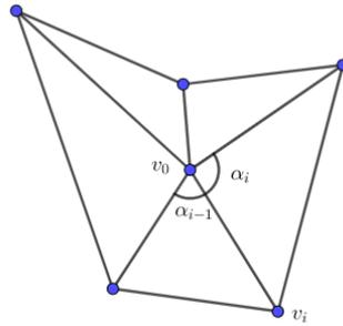
FIGURE 3.4. The mean value coordinate at  $v_0$
