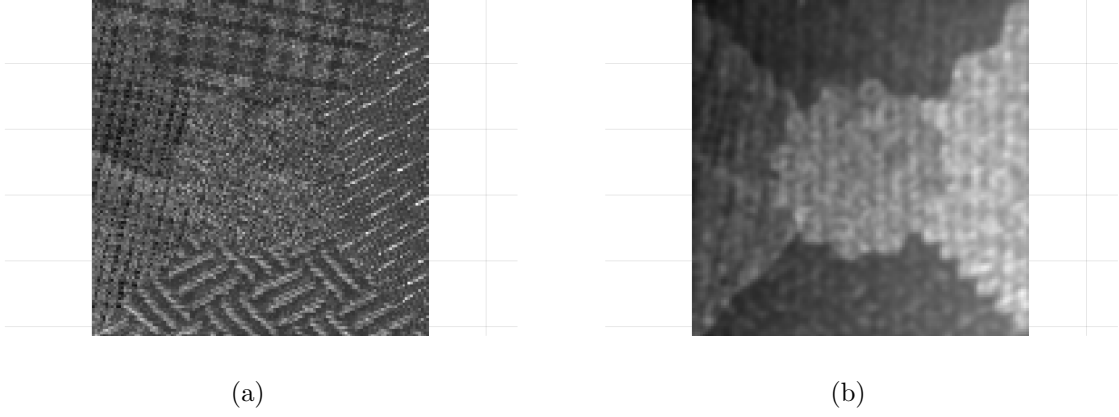
FIGURE 5.9. (a): A composite textured image of size 128 \times 128 ; (b): Mask image computed from PCA of Gabor transform coefficients
