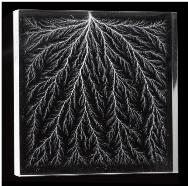
FIGURE 5.2. Lichtenberg figure in perspex block showing fern-like pattern of ionized paths through the material produced by corona discharge from a 2 million volt Van de Graaf electric generator, 1956; courtesy of National Museums of Scotland [1]
